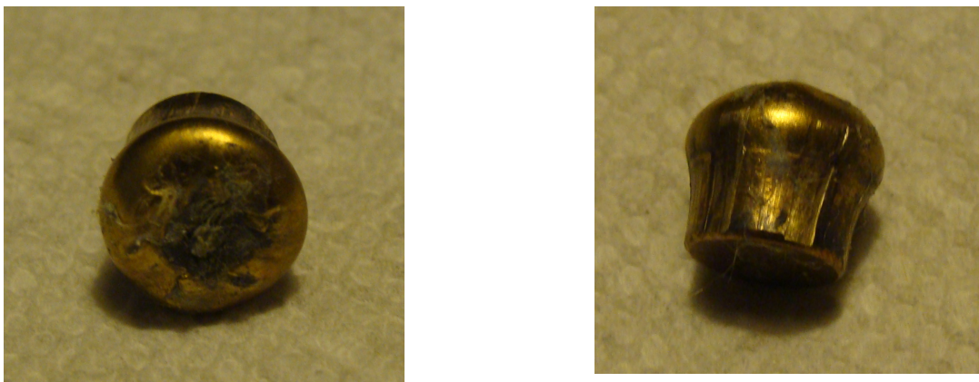
Figure 17. The .380 hollow-point bullet plugged with Kevlar (right) and did not mushroom as much as the .95 grain .380 bullet.
