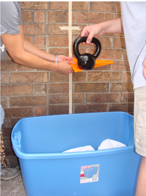
Figure 5. Dropping the weight on the ballistics gel.
