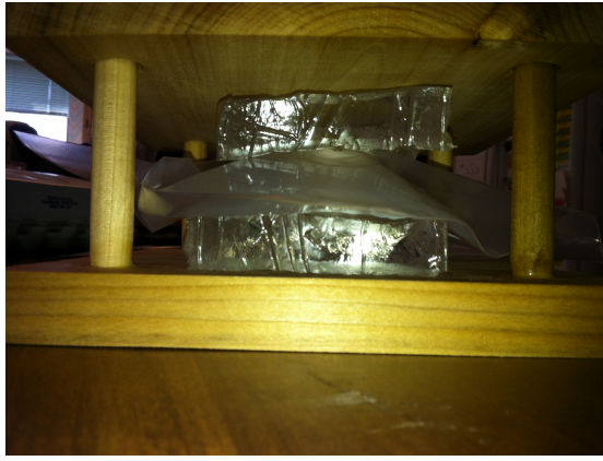
Figure 7. Egg between ballistics gel in egg crusher.
