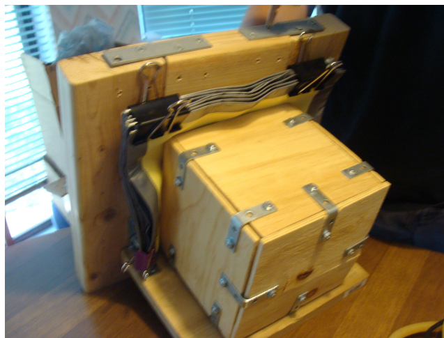
Figure 11. Kevlar layers placed between box and shield.
